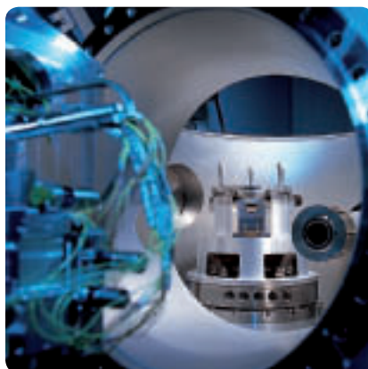
Mirror system for a sample EUV (Extreme Ultra Violet) lighting system for next-generation microchips
