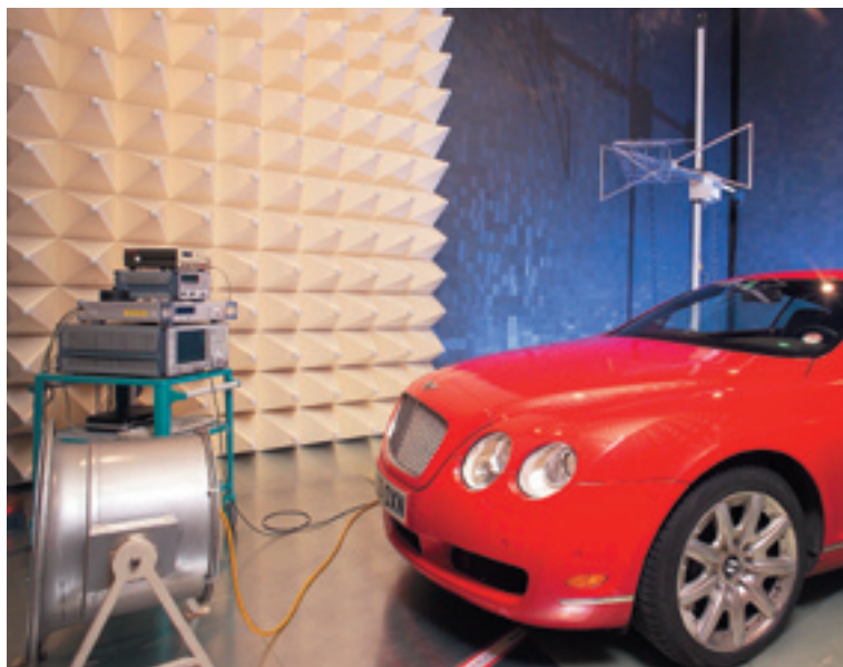
The EMC center is an important component of the BERU RDC. This is where BERU products are tested for their electromagnetic compatibility.
